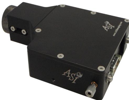
ASI's Continuous Reflective Interface Sample Placement (CRISP) system is designed to maintain focus over time i.e. compensate for thermal & other factors that may cause the sample to drift out of focus over time. It also can be used to maintain a given focal point while scanning the sample in XY. If you are looking to find the optimal focal point while scanning through the sample in Z please see our video autofocus system.
